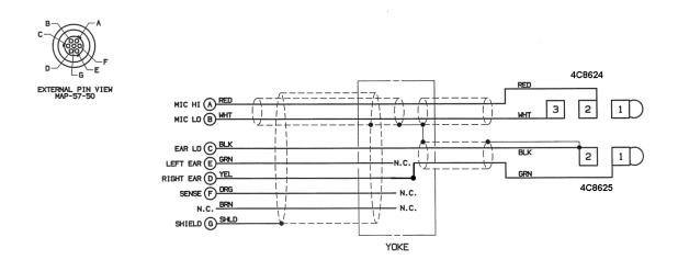
Figure 1: Cable Schematic (41035G-04)
